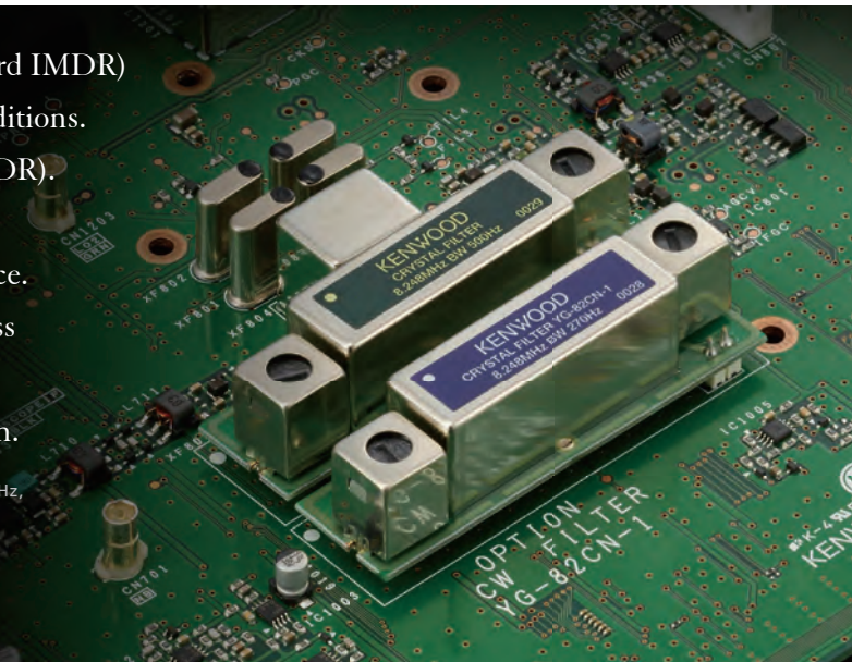
Photograph shows optional 270Hz roofing filter installed.
