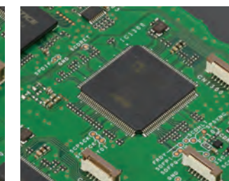
For band scope ADSP-21363 clock @332MHz
